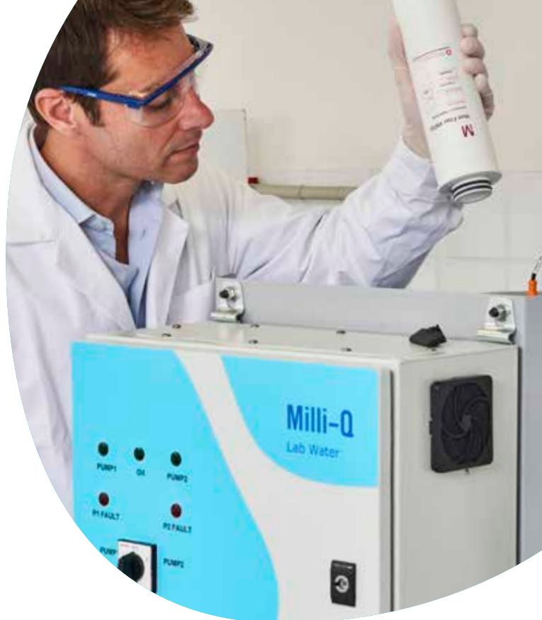
Lab technician changing SDS 500 vent filters
