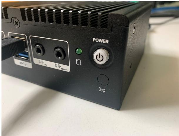
**11. Insert the USB drive into each Assurance® GDS adaptor box one at a time. Ensure the respective Assurance® GDS RGQs are connected to the Assurance® GDS adaptor boxes via USB and are turned on.**
