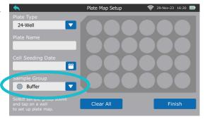
All wells should be assigned to groups for the instrument to recognize them for measurements.
