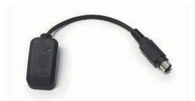
1. Insert the verification adapter device into the instrument port labeled "Sensor" as seen in the picture on the left.
