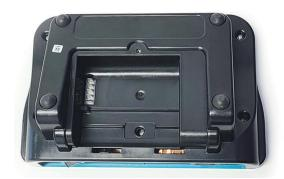
4. To connect a new battery pack to the instrument, line up the battery mating connector on the instrument to the corresponding battery pack connection so that the protruding touch points match (as shown). Push the connector straight down over the pins on the instrument. Do not force the connector; if aligned properly, it should slide into place with little effort.
