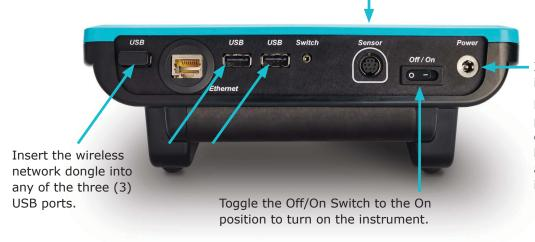
Insert the power cable into the power port.
