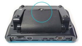
The battery pack is mounted to the base of the instrument. Remove the battery pack from the instrument by pulling up on the battery pack tab. This will decouple it from the instrument and lift the battery pack up.
