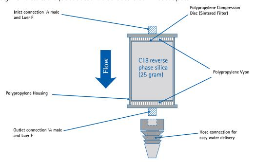
The granular C18 reverse phase silica in the polypropylene housing is tightly packed by a compression disc to avoid any channeling effect. This ensures that the water passing through the LC-Pak® will be in close contact with the C18 chains binding organic molecules by hydrophobic interactions.
