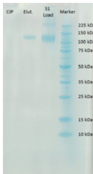
Figure 9. Analytical results of the sample fraction characterization using a SDS-PAGE analytical method displayed in traces of analyzed elution fraction, including loaded glycoprotein (load) at 1 mg glycoprotein/mL CV loading and cleaning (CIP) with 1 M NaOH.
