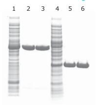
Replicate purification of 38 kDa (lanes 2, 3) and 24 kDa (lanes 5, 6) His-tagged proteins using PureProteome™ Nickel Magnetic Beads. Lanes 1 and 4, corresponding E.coli cell lysates; lanes 2, 3, 5, 6, eluted recombinant proteins.
