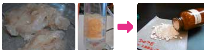
Figure 5. Improvements to the process used to manufacture DOPE enabled production of a free-flowing powder.
