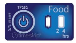
The Timestrip® Food indicator monitors time elapsed at or above 5°C/42°F for up to four hours and stops monitoring it at or below its STOP temperature (3°C/37°F). It is inert until activated and can be stored at room temperature until needed. It is self-adhesive, single use and irreversible. It has a preactivation shelf life of two years from shipping and a one year active shelf-life.
