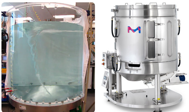
Figure 1. Mobius® Power MIX 1000 prototype tank, used in development, and final production vessel
