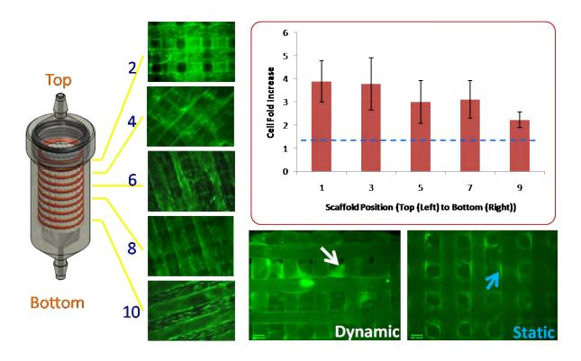
Figure 4.Assessment of cell viability and growth as a function of 3D scaffold position and presence of perfusion at day 6. Cells were viable along the length of the bioreactor chamber (even numbered scaffolds, left image). There was a significant fold increase on odd numbered scaffolds, in comparison to static growth (blue dotted line, top right. Dynamic culture also increases the formation of 3D cell sheets faster than in 3D static (white and blue arrows, bottom right).
