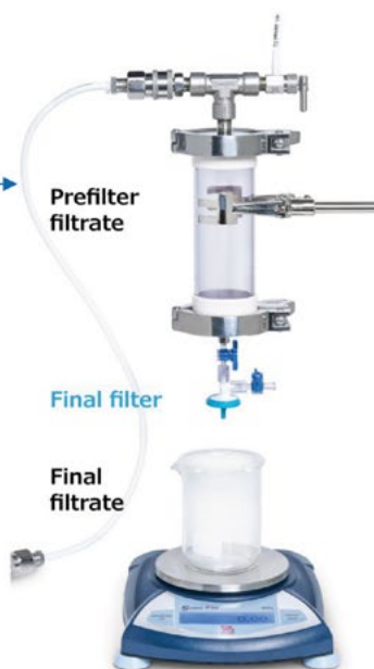
Figure 1. (A) Adsorptive prefilter decoupled from virus filter (B) adsorptive prefilter coupled with virus filter
