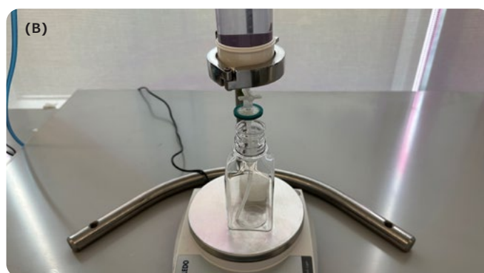
Figure 2. Decoupling prefilter and virus filter can reduce throughput.
