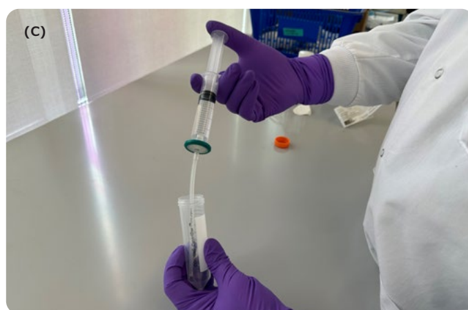
Figure 3. Gentle handling techniques: (A) gravity siphoning, (B) filtration with constant pressure, and (C) microfiltration for monodispersity assessment on a small offline sample.
