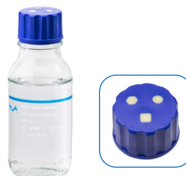
Type 3: Bottle with screw cap with 3 septa. Picture depicts 125 mL bottle with filling volume of 100 mL.
