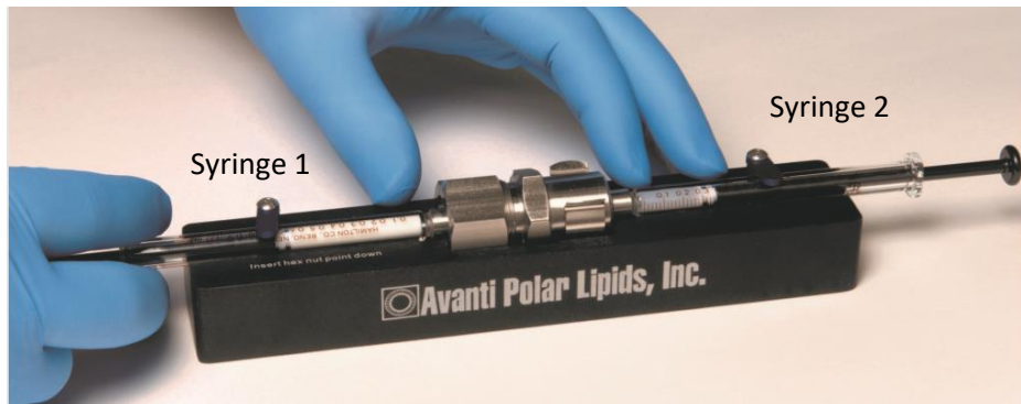
Figure 1. The lipid extrusion process. The MLV solution in Syringe 1 is transferred to Syringe 2 by gently pushing on the plunger of Syringe 1. The solution is then transferred back to Syringe 1 by gently pushing on the plunger of Syringe 2. This process is repeated for a total of 11 cycles.
