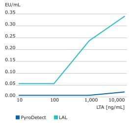
The pyrogenic activity of Lipoteichoic Acid (LTA) is reliably detected with the PyroDetect System. Serial dilution of LTA in the PyroDetect System (red) as compared to the LAL Test (blue). Measured OD values are expressed as Endotoxin Units (EU) per mL referring to an international endotoxin standard.
