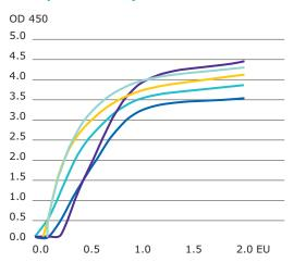
Comparable preparations of the endotoxin standard curve by five users. Different endotoxin dilutions are used in the PyroDetect assay procedure. Quantities of IL-1 $\beta$  are displayed as Optical Density (OD450) against the used concentrations (Endotoxin Units, EU).
