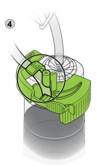
• Grab the tubing and place it in the hook to secure the guide in place and keep the tubing bent. (3–4)
