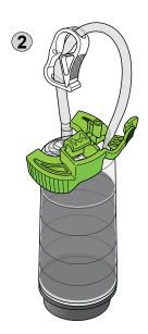
• When sampling is required, transfer the canister in a biosafety cabinet and decontaminate the tubing from the clamp to the chimney. Install the Needle Guide on the top of the canister, around the vent filter. (1) Make sure the tubing is inserted inside the open clamp. (2)
