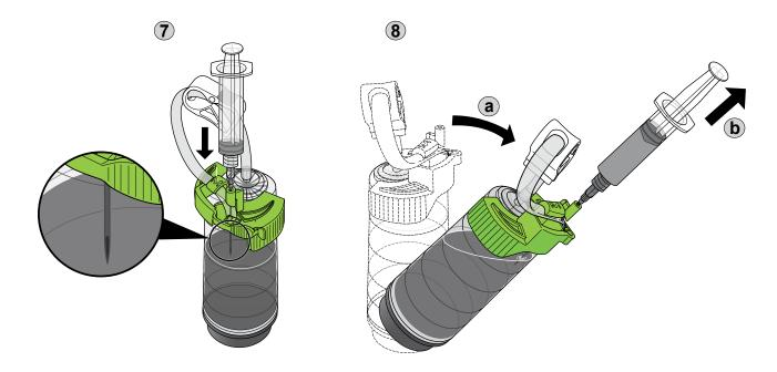
• Once fully down, tilt the canister to access the media and sample. (7–8)
