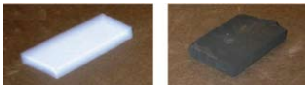
Figure 1. Photographs showing un-doped (left) and carbon-doped (right) ultra-low density \text{SiO}_2 network material.
