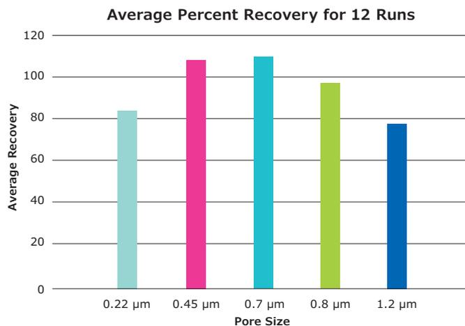
The average performance of each pore size was determined using all the test systems
