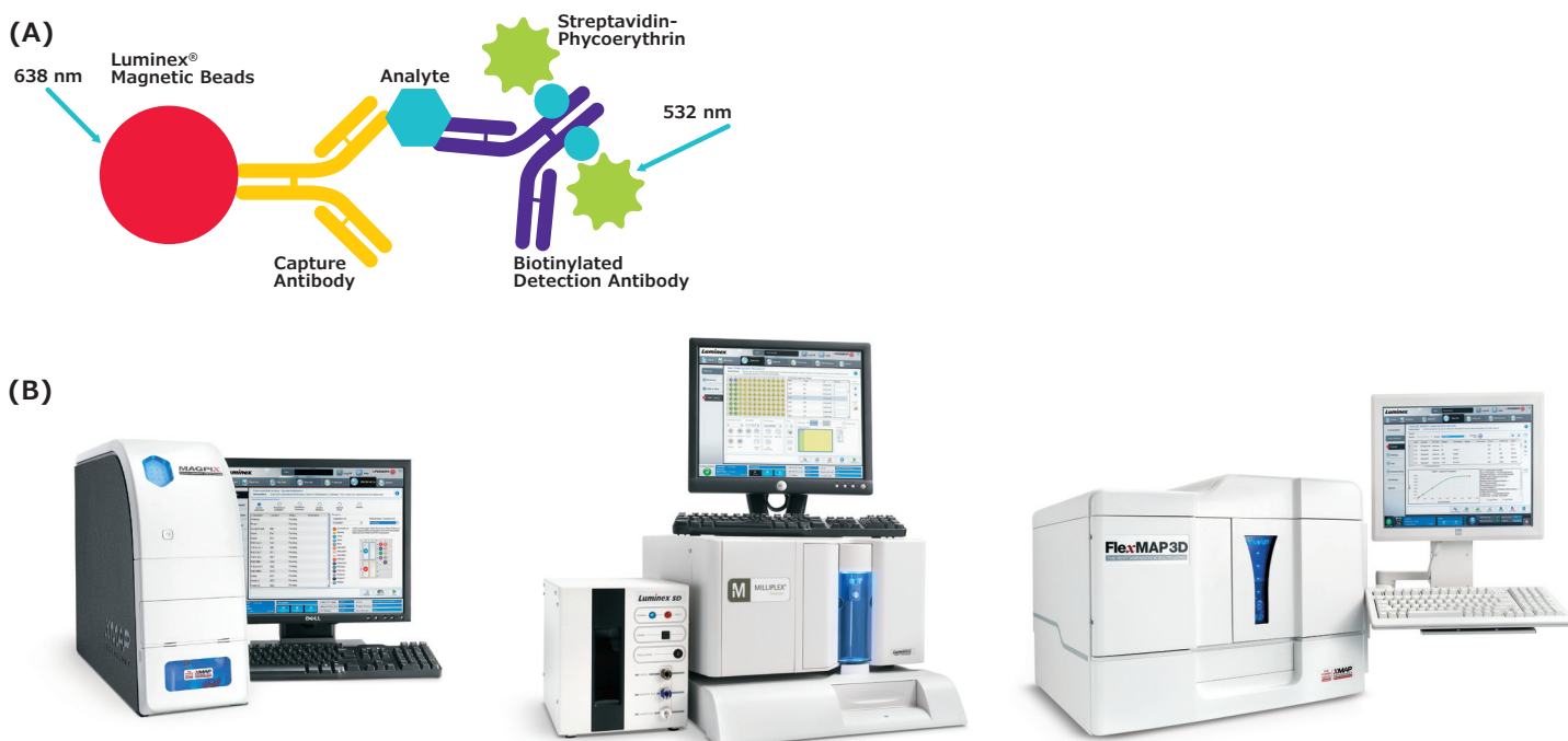
Figure 1. (A) Luminex® protein detection immunoassay method. (B) Instruments for use with MILLIPLEX® kits (left to right: MAGPIX®, Luminex® 200™, FLEXMAP 3D®).
