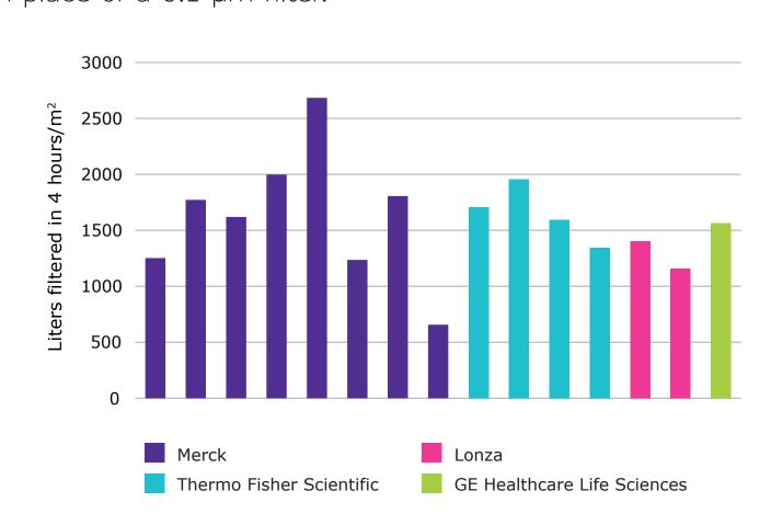
Viresolve® Barrier filter shows high capacity for efficient filtration of most commercially available chemically defined media.
