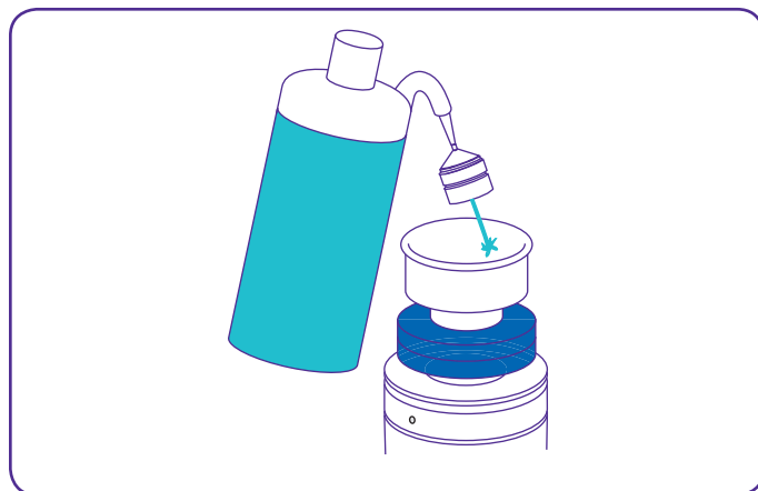
Figure 30. Wash down inside of funnel.
