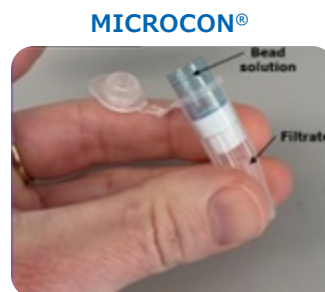
Figure 4: Image of a Microcon ® centrifugal device used for testing hydrophobic PP membrane filters
