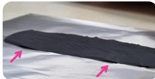
Figures 6.1 to 6.4. Representative images of electrodes fabricated under non-optimized slurry conditions, illustrating defects such as (6.1) cracking, (6.2) layer separation, (6.3) insufficient coating, and (6.4) delamination. All samples were prepared under identical coating and drying conditions, highlighting the importance of controlling slurry composition and processing parameters for reproducible, high-quality electrodes.
