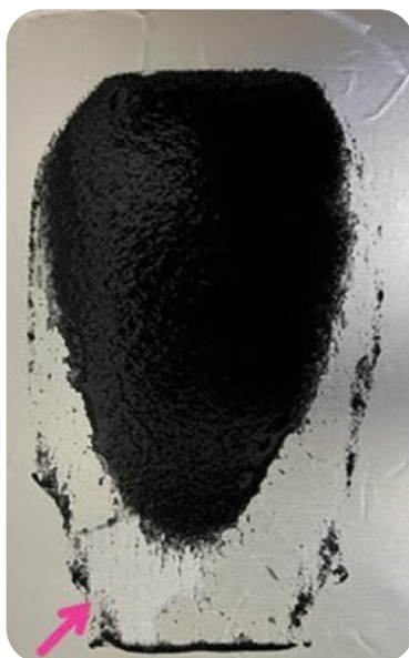
Figures 6.1 to 6.4. Representative images of electrodes fabricated under non-optimized slurry conditions, illustrating defects such as (6.1) cracking, (6.2) layer separation, (6.3) insufficient coating, and (6.4) delamination. All samples were prepared under identical coating and drying conditions, highlighting the importance of controlling slurry composition and processing parameters for reproducible, high-quality electrodes.
