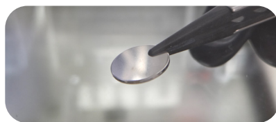
Figures 4.1 to 4.4. (4.1) Photograph of individual components used in the assembly of a 2032 coin-type battery cell, (4.2) NMC811 cathode, (4.3) Li Metal anode, and (4.4) separator.
