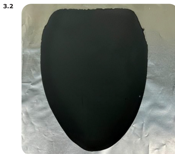
Figures 3.1 and 3.2. Electrode fabrication images: (3.1) Cathode coated using the optimized 35 wt% slurry, demonstrating appropriate areal loading and a uniform, defect-free layer with complete coverage. (3.2) Same electrode after drying and calendering, showing a smooth and compact surface morphology, confirming ideal viscosity and mixing conditions for reliable electrode preparation.
