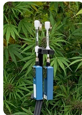
Outdoor measurement of terpenes from hemp growing operations using our glass and stainless steel Carbotrap® T420 TD tubes and Spectrex PAS-500 Personal Air Sampling pumps
