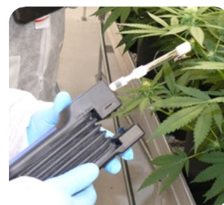
Indoor profile measurement of cannabis terpenes (flowering plant) from cannabis greenhouse growing operations using our glass Carbotrap® T420 TD tubes and detector tube pump
