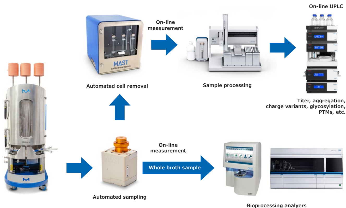
Figure 1: Example workflow for a non-GMP laboratory using the MAST® Autosampling Solution for automated on-line sampling and analysis to support rapid process development.
