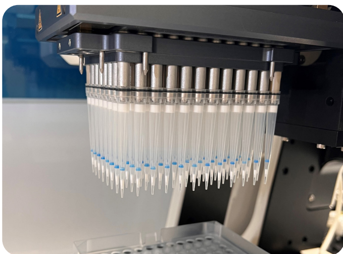
Figure 1. Supel ™ Swift DPX HLB 3 mg (bed) Tips. The tips are being actively picked up by the automated liquid handler.
