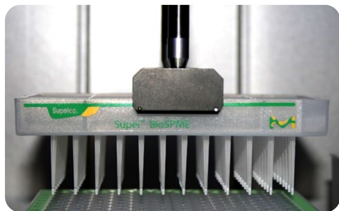
Figure 2. Supel™ BioSPME 96-Pin Device Maneuvered by Automated Liquid Handling System Gripper.
