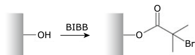
Figure 4. Introduction of ATRP initiator sites onto a hydroxyl-functional surface (e.g., cellulose) using 2-bromoisobutyryl bromide (BIBB).
