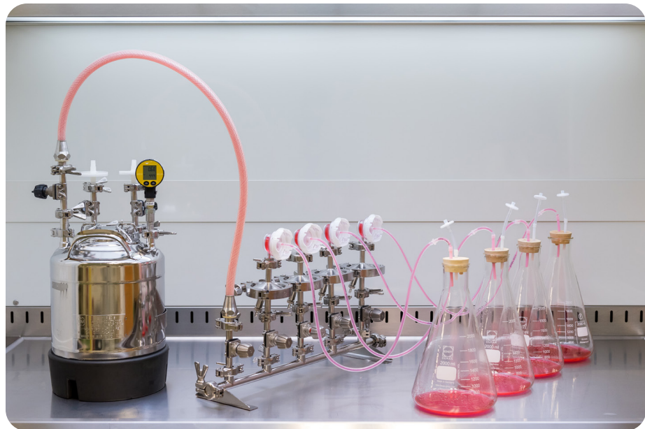
Figure 1. Small scale filter test set-up.
