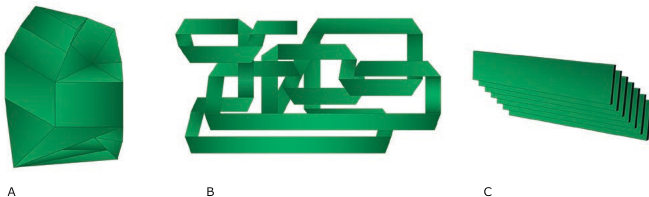
Figure 3. A) Zoomed in illustration of the different graphitic planes on the top surface of PGC. B) The intertwined graphitic ribbons that give PGC particles its robust strength. C) A cut section of a graphitic ribbon exposing multiple layers.
