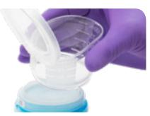
Effortless funnel separation: a simple pinch and the funnel is removed from the membrane: no forceful cracking of the plastic. The funnel lid closes the media plate which is then ready for incubation.
