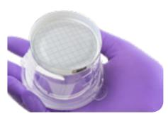
Optimal, touch-free membrane to culture media transfer: the touch-free design includes a sealed membrane that forms a convex shape to avoid bubbles or furled filters for any operator.
