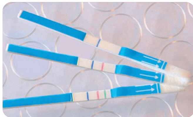
Figure 3 Lateral flow tests using Estapor® Dyed Microspheres (reference: K1-030 blue for the control, K1-030 red and K1-030 green for the analytes) and Millipore Hi-Flow™ membrane.
