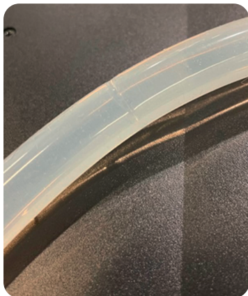
Figure 10. Impact of pinch valves on the tubing.
