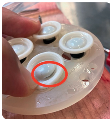
Figure 12. Pump chamber diaphragm failure.
