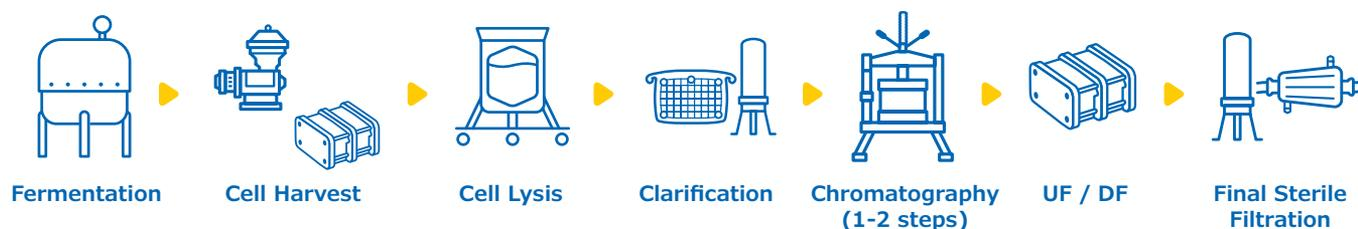
**Figure 1:** General process flow for pDNA manufacturing
