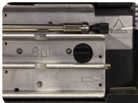
Figure 2. Zoomed-in picture of the column connected properly to the inlet tubing.
