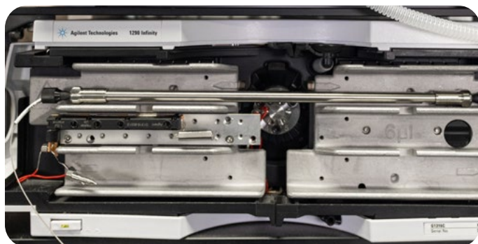
Figure 1. Supelco ® analytical HPLC column installed onto an Agilent ® 1290 U/HPLC instrument. Notice how the column comfortably fits into the column oven.
