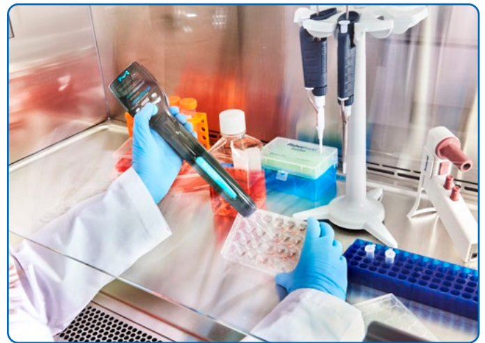
Figure 9. Scepter™ 3.0 handheld cell counter.
