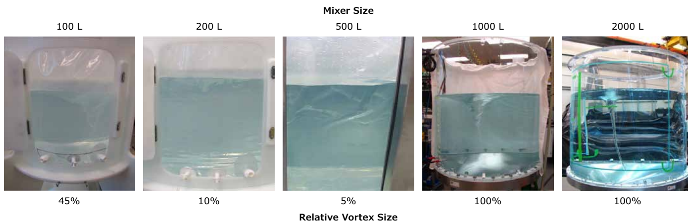
Figure 9. Vortex at 80% volume, maximum speed in Mobius® Power MIX from 100 L to 2000 L.
