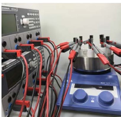
Figure 4. Typical Multicell Setup for Galvanostatic Electro-Organic Transformations (Available as IKA® Screening System for Electrosynthesis).
