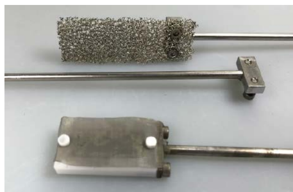
Figure 13. Modified Electrode Holders for Porous Electrode Materials such as Nickel Foam. Front: Stainless-Steel Electrode Holder with Teflon® Frame for Mounting Meshes. Center: Back Side of the Stainless-Steel Electrode Holder for Mounting Foams. Back: Electrode Holder for Foams with Mounted Electrode.
