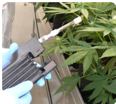
Figure 3. Indoor profile measurement of cannabis terpenes (flowering plant) from cannabis greenhouse growing operations using a glass Carbotrap® T420 TD tube and detector tube pump.
