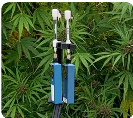
Figure 2. Outdoor measurement of terpenes from hemp growing operations using a glass and a stainless steel Carbotrap® T420 TD tube and a Spectrex PAS-500 Personal Air Sampling pump.
