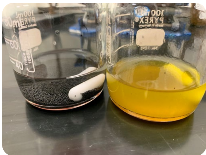
Figure 1. Carboxen® 564 (left) and Silica-Thiol (right) in methanol after a [\text{Rh}(\text{COD})\text{Cl}]_2 scavenging experiment. The discoloration observed with the Silica-Thiol treated solution is the result of the particles suspended in the solution. Carboxen® 564 quickly settles, as can be seen by the black layer under the stir bar.
