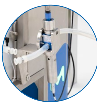
Pre-column instrumentation for conductivity and pH measurement
