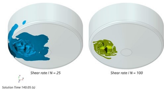
Figure 7: Dimensionless shear rate (25; 100) at 54 L and 150 rpm.
