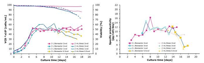
Overall, the data shows broad comparability between the Mobius® Breez Microbioreactor and the 3 L benchtop reactor, indicating Mobius® Breez is a suitable scale-down model for perfusion performance predictability. The data also showcases the benefits of running perfusion, which allows for several experiments to be performed in the same run, thus saving time. In this instance, the experiment shifted from 2.0 VVD to 1.0 VVD on day 8 and then to 0.5 VVD on day 12.
