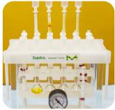
Multiple Sample Elution w/Vacuum Manifold, 12-Port (Cat. No 57044)
