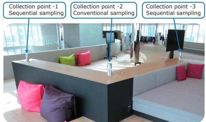
Figure 2. Photo of the three air sampling locations for Part 2. The distance between the sampling locations was approx. three meters.
